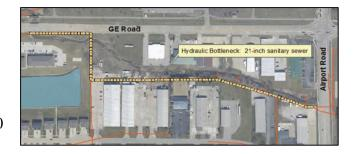
inches down to 21 inches. The 21-inch sewer is substantially undersized. Options are under review to increase capacity of the Hawthorne Collector Sewer.
