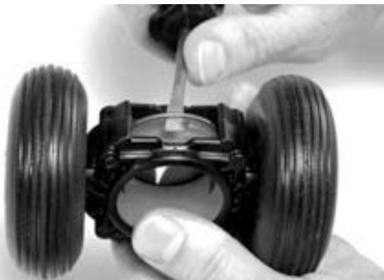
Figure 20 – Opening The Roller Dolly Retaining Rings
