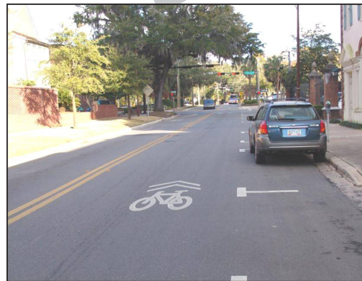
Figure V-3. Sharrows in Use in Tallahassee, FL
