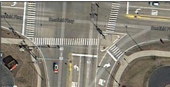
Figure 2.4. Top: Bringing sidepath crossings closer to the parallel road. Bottom: Right-turn corner island and high-visibility continental crosswalks
