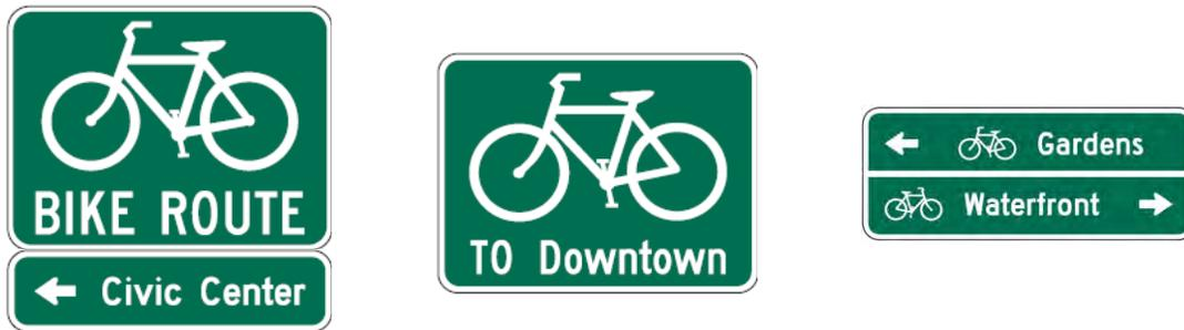
Figure 2.10. Bike Route wayfinding sign options. Left: D11-1/D1-1 Middle: D11-1c Right: D1-2b
