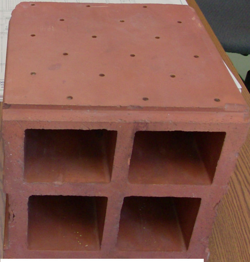
B. Existing underdrain to be replaced
