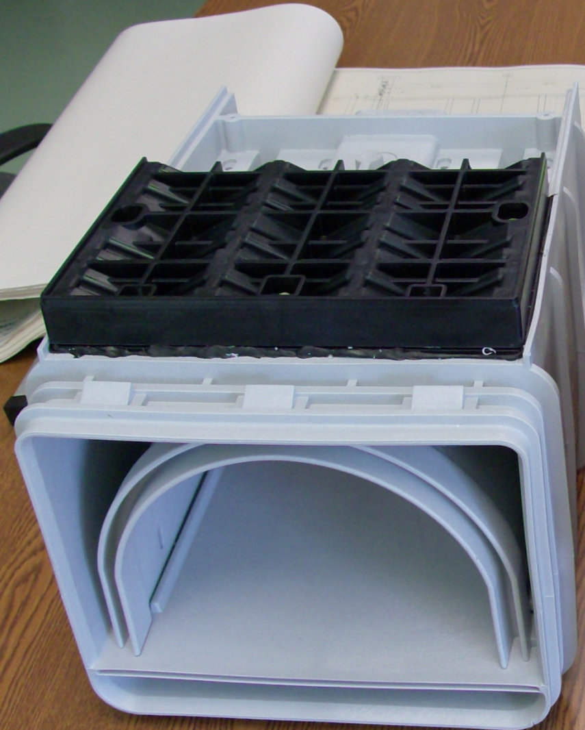
A. Proposed new gravel-less underdrain
