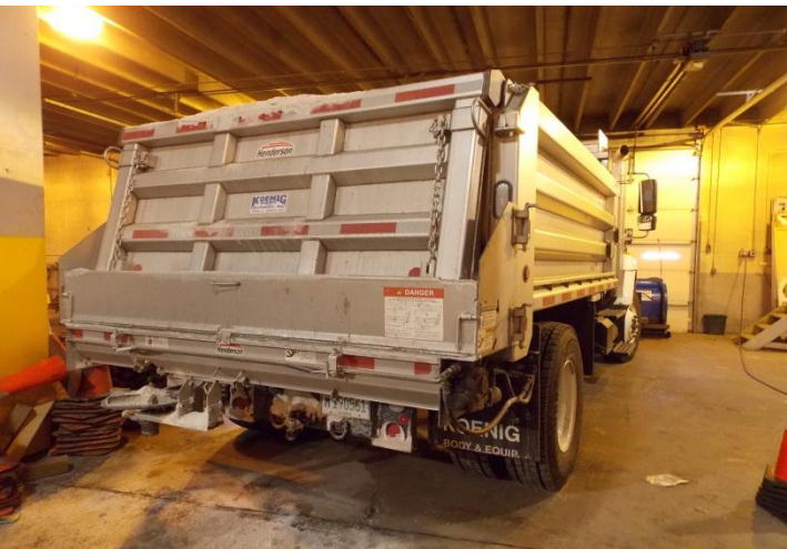
Spreader Mounted on Truck for Snow Event
