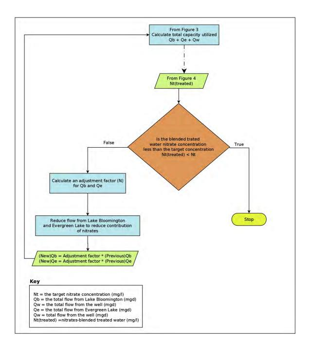
Figure 5: The iteration process used in the Treatment Model.
