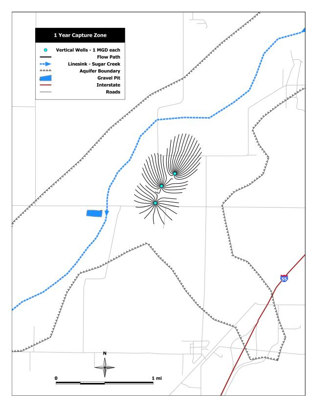
Figure 47: Simulated 1-year capture zone for Scenario 1 - three vertical wells near the test well with an aggregate pumping rate of  $3 \, mgd$ . Stream resistance is  $1 \, day$ .
