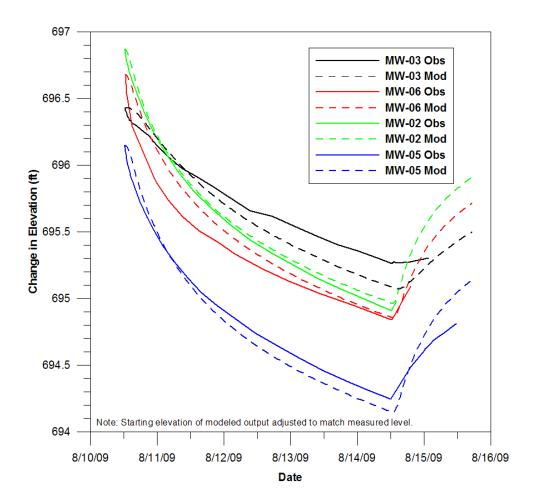
Figure 39: MODFLOW model calibration results.
