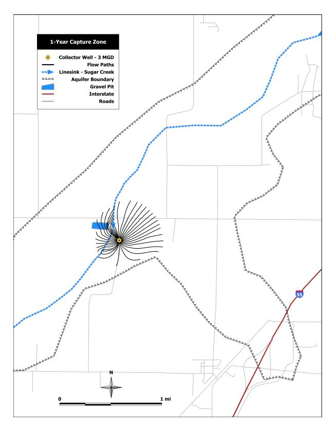
Figure 49: Simulated 1-year capture zone for Scenario 3 - one collector well south of the test well along Sugar Creek with a pumping rate of  $3 \, mgd$ . Stream resistance is  $1 \, day$ .
