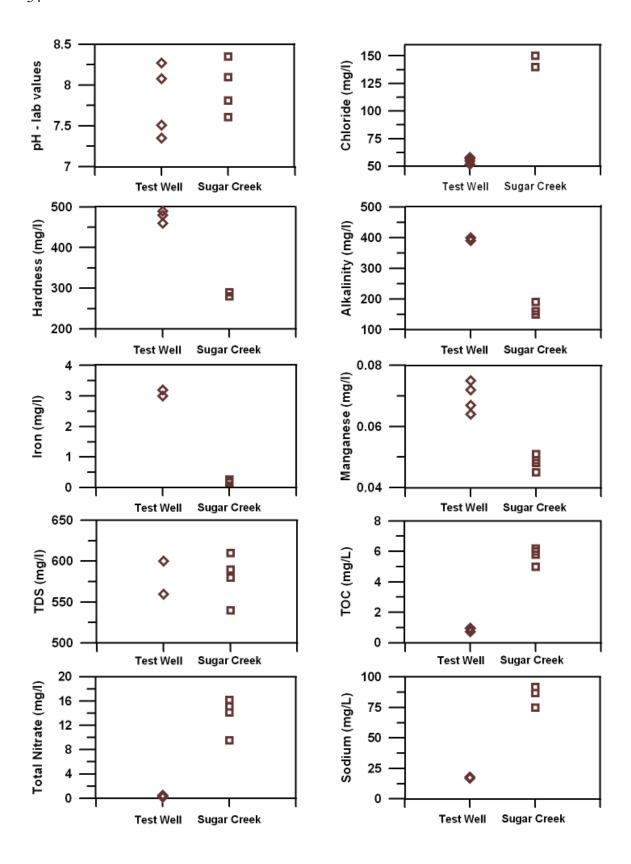
Figure 30: Select water-quality results from the test well and Sugar Creek.
