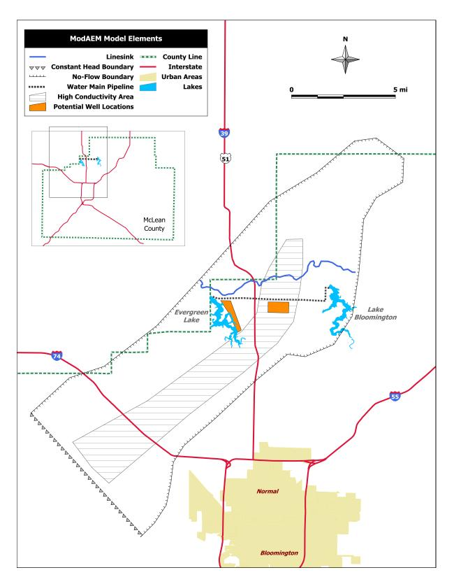
Figure 16: Potential well locations and layout of ModAEM groundwater flow model, Danvers Bedrock Valley.
