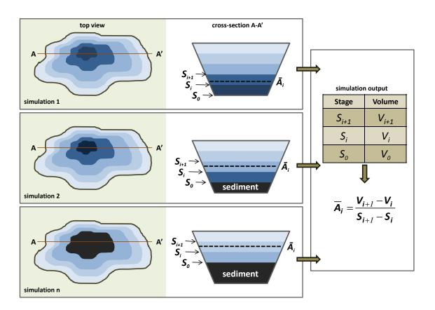
Figure 3: Using the stage-volume table to estimate lake surface area and volume during the simulation.
