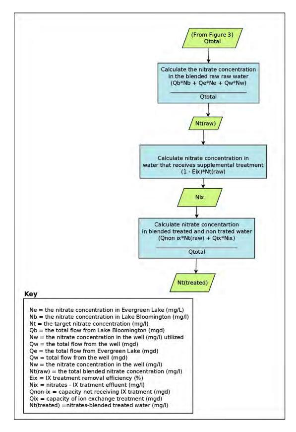
Figure 4: The process used in the Treatment Model to calculate the nitrate concentration of the blended water.
