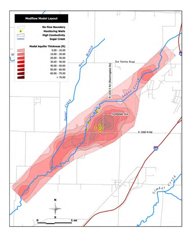
Figure 38: Layout of MODFLOW model of Sugar Creek Aquifer.
