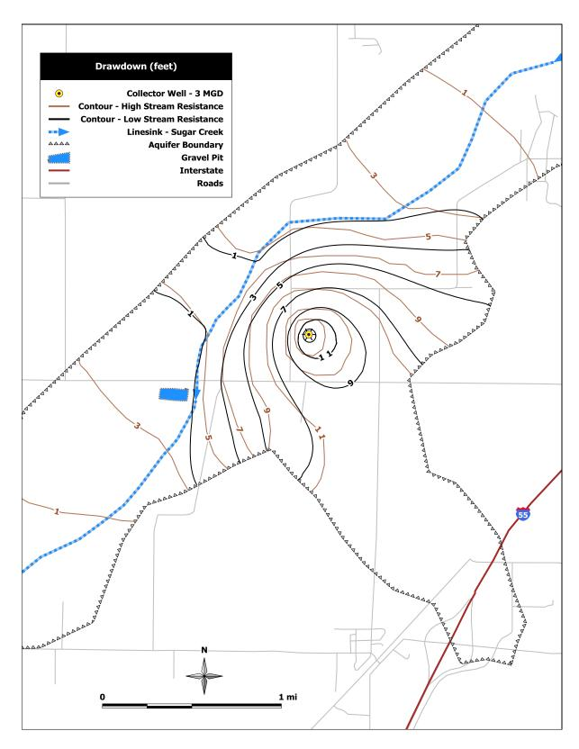
Figure 44: Simulated drawdown distribution for Scenario 2 - one collector well near the test well with a pumping rate of 3 mgd. Black contours are for 1 day stream resistance and brown contours are for 5 day stream resistance.
