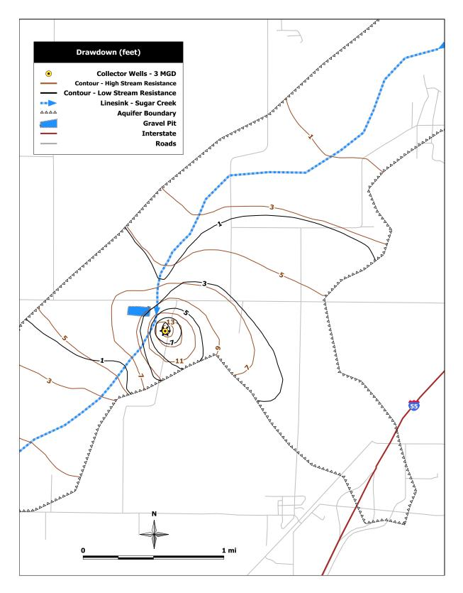
Figure 45: Simulated drawdown distribution for Scenario 3 - one collector well south of the test well along Sugar Creek with a pumping rate of 3mgd. Black contours are for 1day stream resistance and brown contours are for 5day stream resistance.
