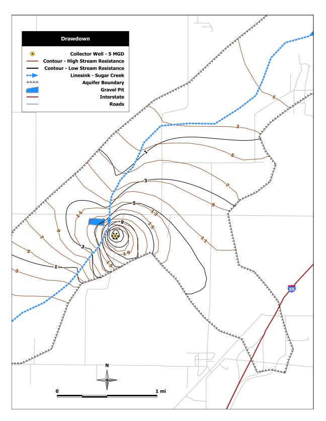
Figure 46: Simulated drawdown distribution for Scenario 4 - one collector well south of the test well along Sugar Creek with a pumping rate of  $5 \, mgd$ . Black contours are for  $1 \, day$  stream resistance and brown contours are for  $5 \, day$  stream resistance.
