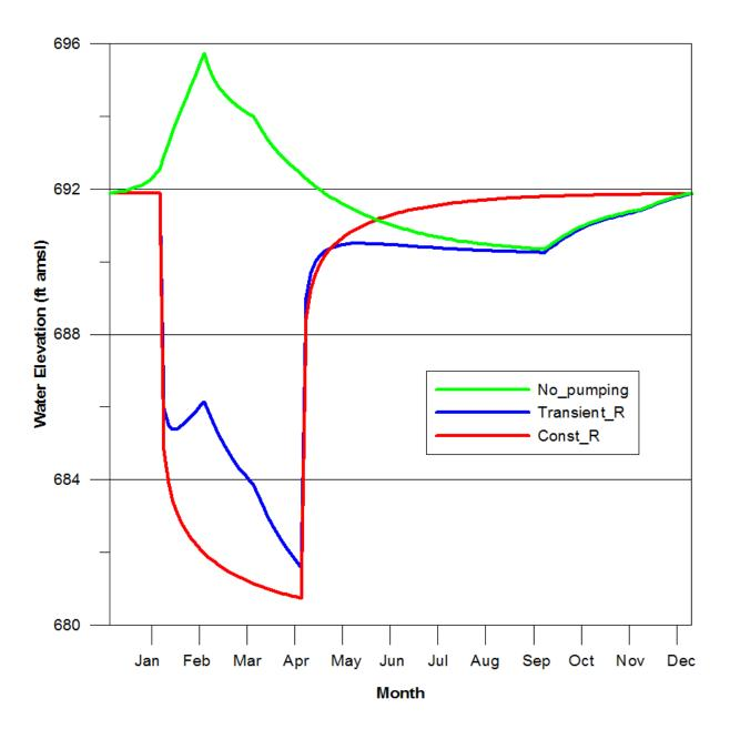
Figure 40: Simulated annual variation in groundwater level at the location of the test well.
