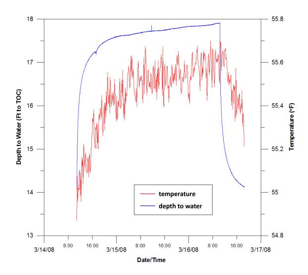
Figure 25: Results of aquifer test at Fox Creek Golf Course: drawdown and temperature recorded at the monitoring well.
