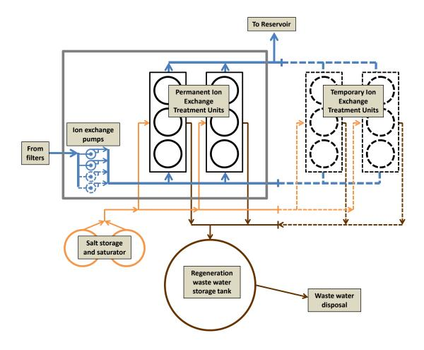
Figure 5.4: Conceptual process schematic of ion-exchange treatment for nitrate removal.
