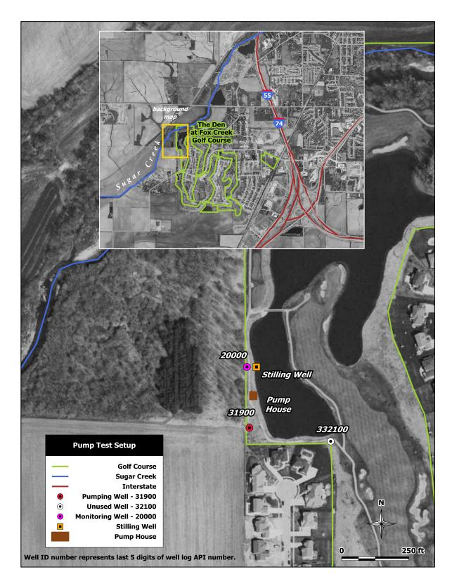
Figure 24: Setup for the aquifer test at Fox Creek Golf Course.
