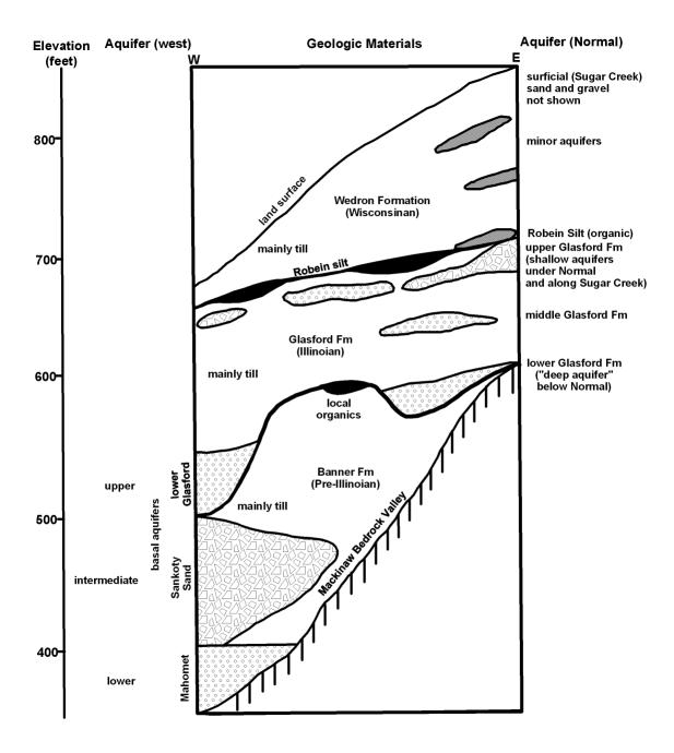
Figure 3: Generalized cross-section of a bedrock valley in the vicinity of Normal, Illinois [Kempton and Visocky, 1992].
