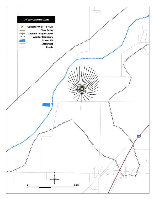
Figure 48: Simulated 1-year capture zone for Scenario 2 - one collector well near the test well, with a pumping rate of  $3 \, mgd$ . Stream resistance is  $1 \, day$ .
