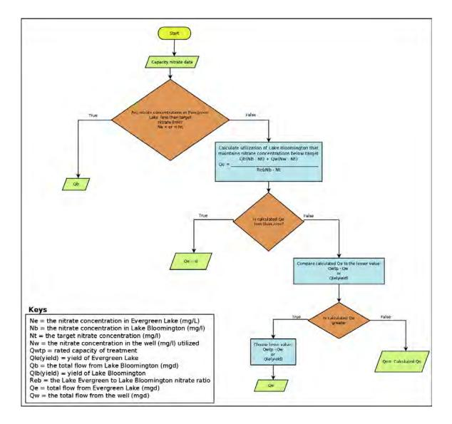
Figure 1: The process used to calculate Evergreen Lake's capacity in the Source Blending Model.
