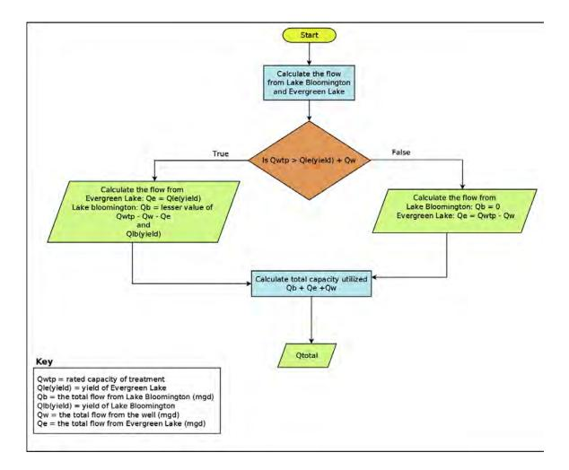
Figure 3: The process used in the Treatment Model to calculate total capacity utilized from Lake Bloomington, Evergreen Lake, and the production wells.
