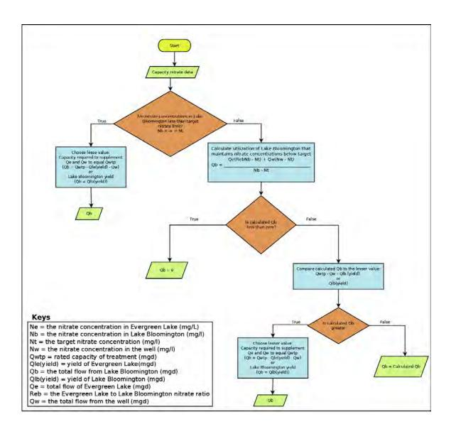
Figure 2: The process used to calculate Lake Bloomington's capacity in the Source Blending Model.
