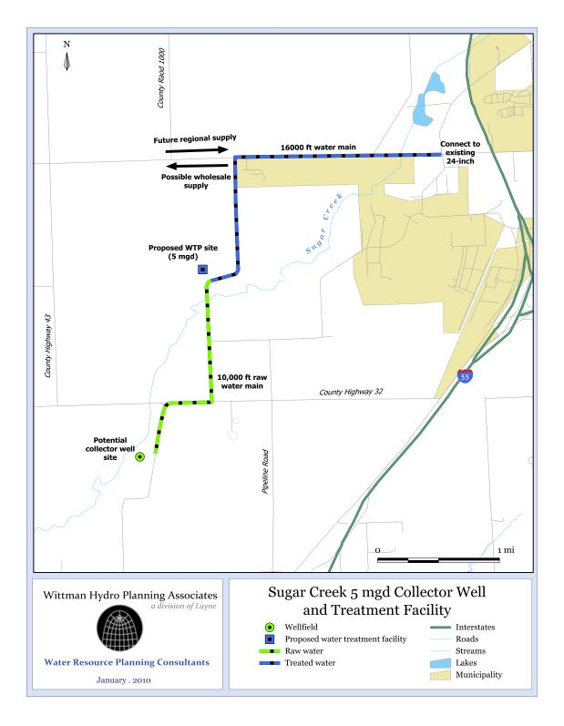
Figure 5.8: Sugar Creek 5 mgd collector well and treatment facility.
