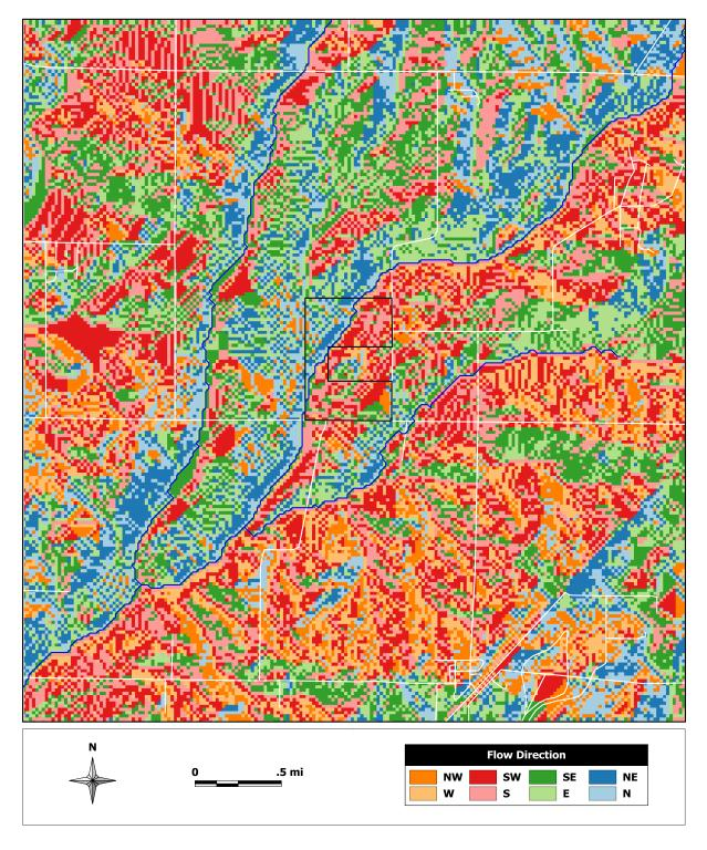
Figure 35: Flow direction of runoff [USGS, 2001].
