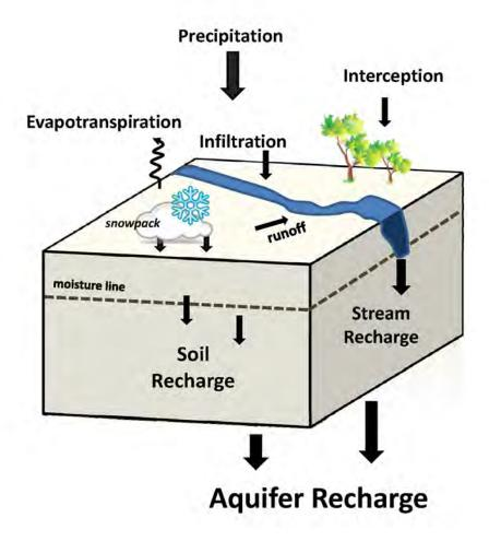
Figure 31: Conceptual model of the soil-water balance.
