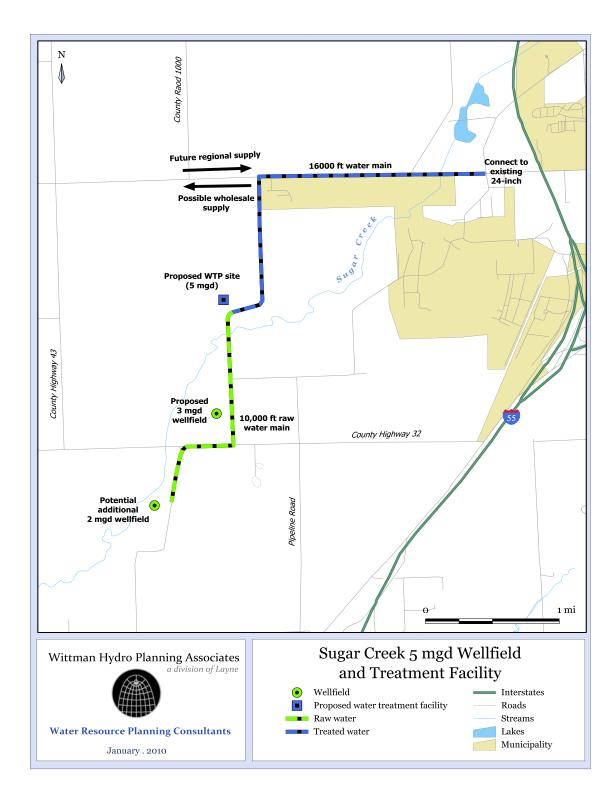
Figure 5.7: Sugar Creek 5 mgd wellfield and treatment facility.
