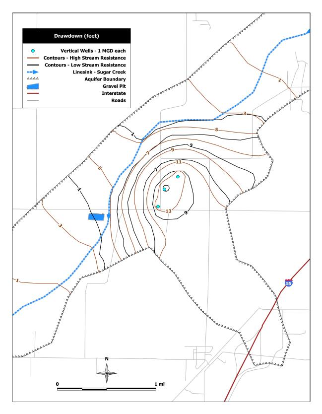
Figure 43: Simulated drawdown distribution for Scenario 1- three vertical wells near the test well with aggregate pumping rate of 3mgd. Black contours are for 1day stream resistance and brown contours are for 5day stream resistance.
