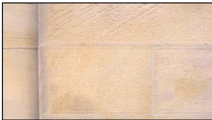
Limestone – A sedimentary rock; used for building walls, window sills and lintels, ornamental stone trim, sculpture and for producing lime.
