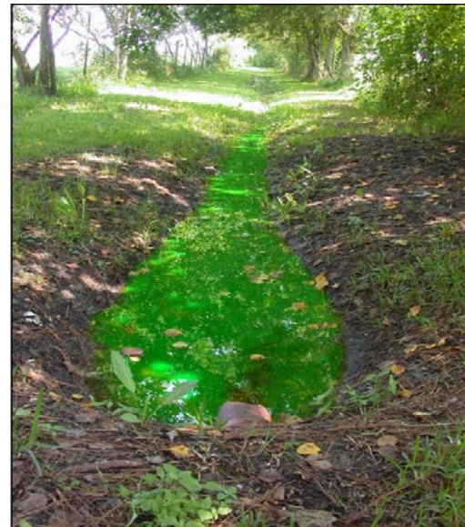
Figure 6. Biodegradable dye has been detected in nearby water, indicating septic system failure. 18
