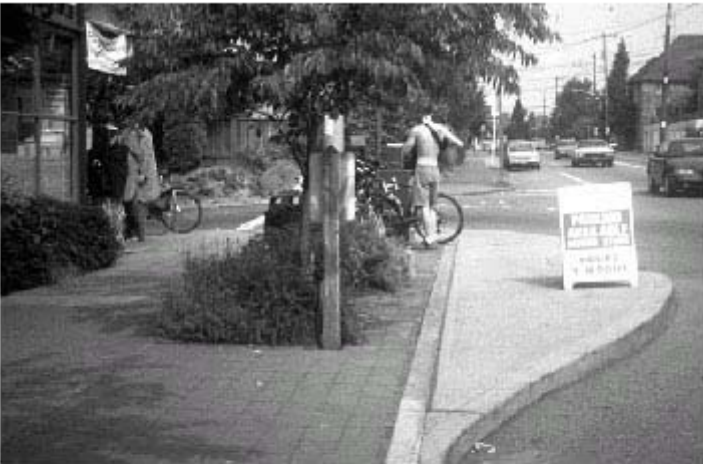
A curb extension on an arterial street in Seattle, Washington. The crossing distance for pedestrians is substantially reduced by the installation of this device.
