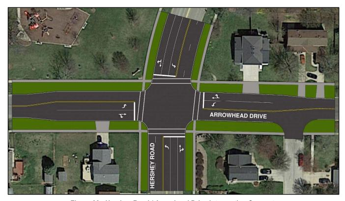
Figure 22 - Hershey Road / Arrowhead Drive Intersection Concept
