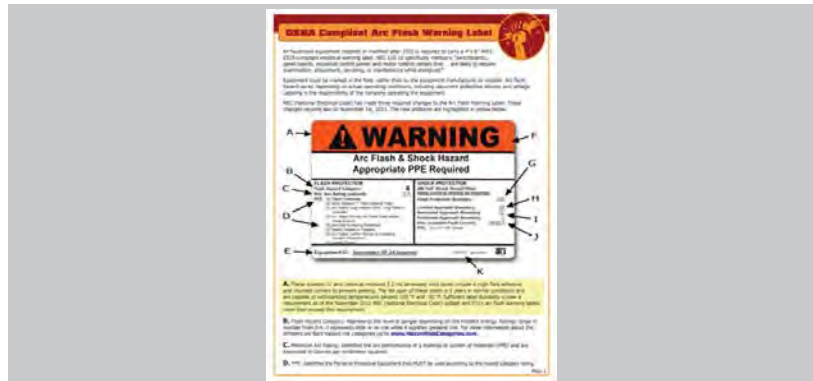
Example arc-flash warning label.
